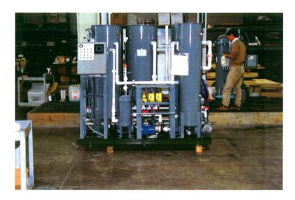
Waste water treatment plant for oil & grease, heavy metals & COD removal. The system is a fully automatic waste water recycler. The treatment plant is very effective in removing oils, grit & grime, etc. from automatic car washers, steam cleaners, etc. The system maintains a proper pH balance and removes bacteria. The waste separated is a semi-dry cake.
