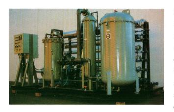
EEC Waste-sep is an industrial membrane separator for a wide variety of chemically or mechanically emulsified solutions. EEC Waste-sep uses advanced technology with proven concepts in efficient oil & water separation techniques. The result is a fully-automatic liquid separator that can condition a milky, emulsified solution of oil, chemicals, ink, cutting oil & diesel fuel to its origin.
